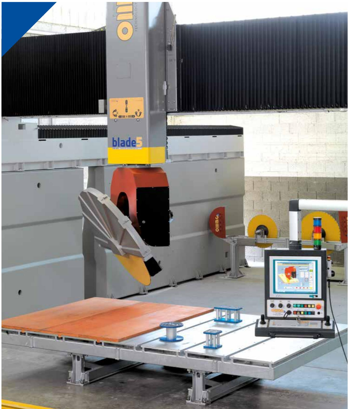
**BIROTAIRY** blade head for cross, circular and inclined cuts sawblade Ø 800÷1.600 mm
